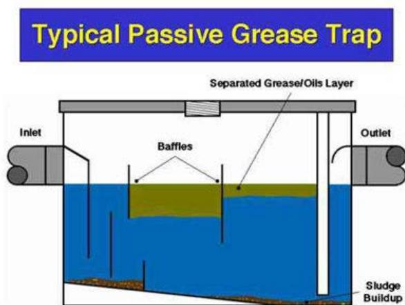
A grease trap looks like a large box or barrel spliced into the water drainage line. When the water enters the grease trap, it cools down, allowing the lighter oil to precipitate out to the top. A series of baffles in the grease trap collect oil and chunks of material while the water sinks to the bottom. An exit pipe at the base of the grease trap allows the treated water to flow out, while the grease remains enclosed on top.
